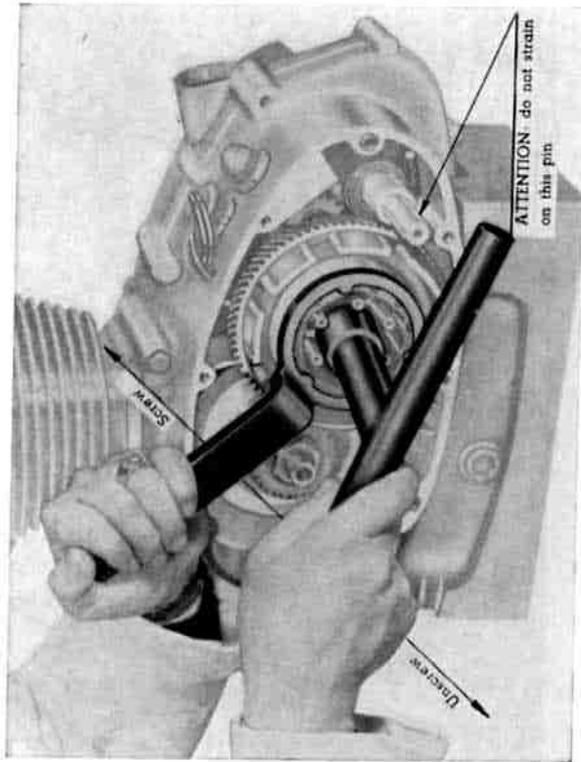
5 - Spanner to secure the clutch drum
